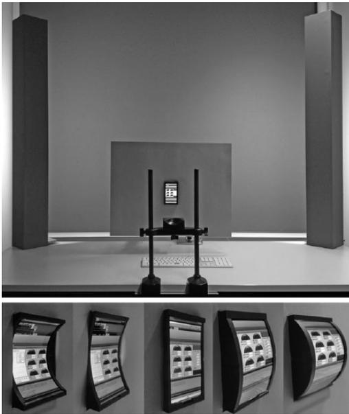
Figure 2. Experimental setup and display curvatures. Curvatures from left to right are *high concave* ( $r = -50$  mm), *low concave* ( $r = -100$  mm), *planar*, *low convex* ( $r = 100$  mm), and *high convex* ( $r = 50$  mm).
